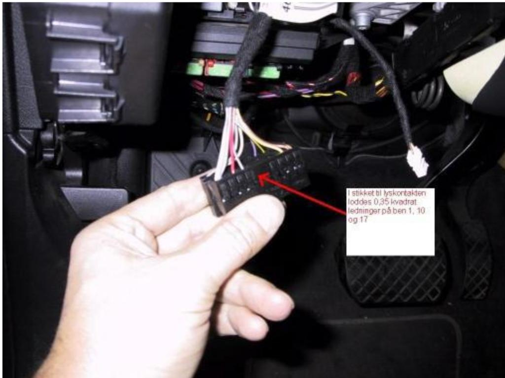
(Here you should solder/attach the cable on pin 1, 10 and 17)
